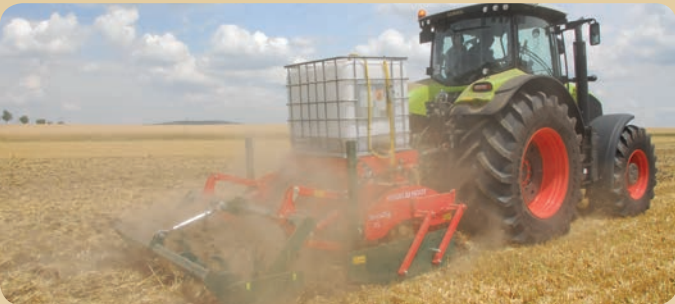
Subsoiler with spray equipment for BB Soil
